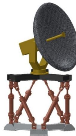
Fig. 2. Antenna on a six-axis motion simulator.
