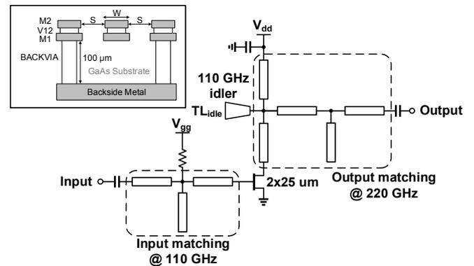
Fig. 3. Schematic of the G-band frequency doubler.
