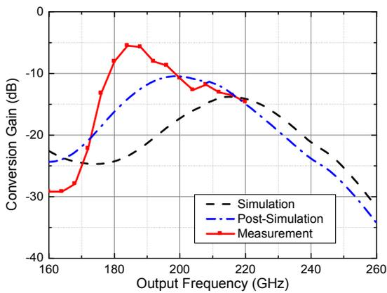
Fig. 9. Measured conversion gain at  $P_{in} = -16$  dBm.
