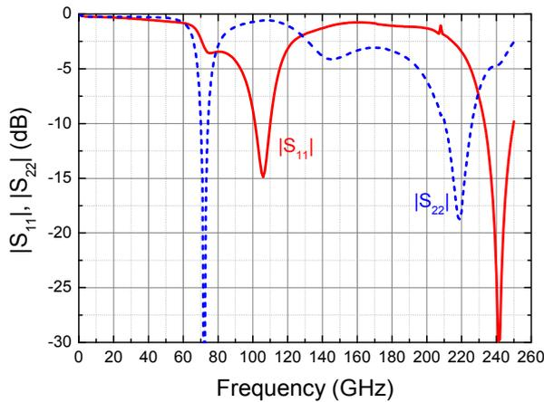
Fig. 5. Simulated input and output matching performance.
